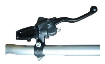
12. Insert the bladder (12) back in the reservoir. Place the cap (11) and tight the screws (10) with a torque wrench with TX20 tool with 1.25±0.25 Nm torque.
