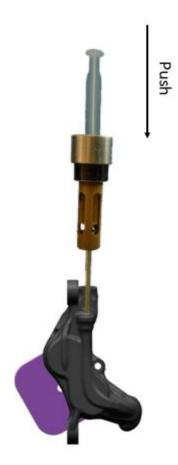
8. Remove the old oil present in the master cylinder reservoir using a syringe.
