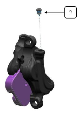
14. Clean the caliper and the mastercylinder from any oil residual with brake cleaner and wipe with a cloth.
