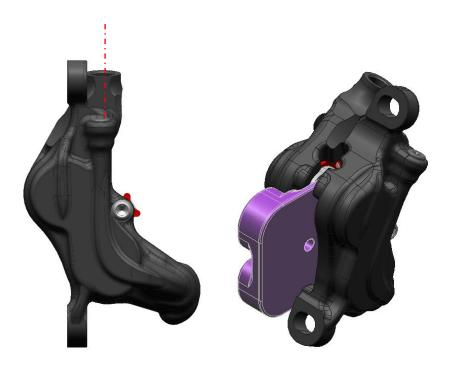
2. Remove the bleeding screw (9) with a Torx T10 key.
