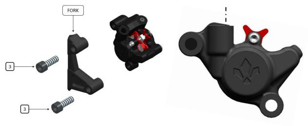
2. Remove the bleeding screw (8) with a Torx T10 key
