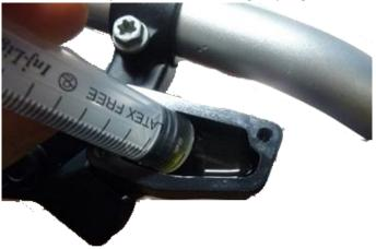
9. Pour some new DOT4 oil from a sealed bottle in the master cylinder reservoir.
