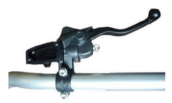
12. Insert the bladder (11) back in the reservoir. Place the cap (10) and tight the screws (9) with a torque wrench with TX20 tool at 1.25±0.25 Nm.
