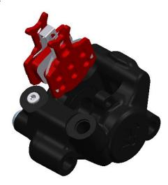
5. Insert the pin (5) and tight it with a torque wrench with HEX 3 mm tool at 2±0.25 Nm. Place the seeger (4) in its seat.
