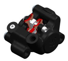
14. Clean the caliper and the mastercylinder from any oil residual with brake cleaner and wipe with a cloth.
