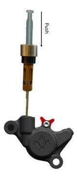
8. Remove the old oil present in the master cylinder reservoir using a syringe.
