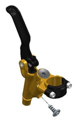
4. Unscrew the lever pivot (7 and 8). Remove the dust seal (9) and the seeger (10), so that the lever and the pushrod can be removed.
