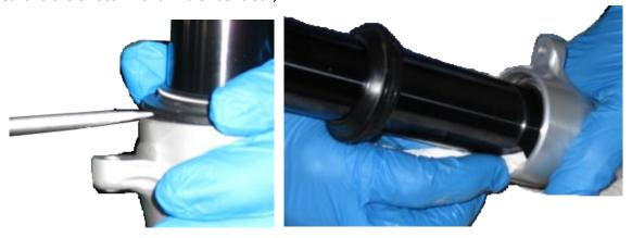
3. Insert a microfiber cloth inside the dust seal to remove dirt residue from the internal diameters, then apply grease on the tube;
