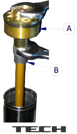
4. Keep the cap (C) inside the cartridge stem. Remove all the oil inside the cartridge by moving up and down the stem and dispose of it according to local laws. Tighten the wheel's axle in a bench wise with aluminium plates and insert the leg on the axle;
