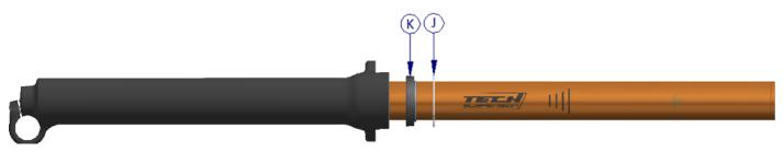
17. Apply grease in the highlighted area. Rotate the dust seal (J) on the grease and insert the dust seal in its housing by pushing on its outer diameters with a screwdriver;
