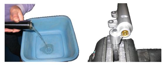
8. Push the tube inside the leg (end stroke) and insert Tool 3 inside the tube to disassemble the pumping stem (G), then unscrew the regulator for the end stroke (F) with a 12 mm hexagonal key;
