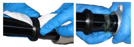
4. Rotate the dust seal on the grease and insert the dust seal in its housing by pushing on its outer diameters with a screwdriver;
