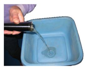
7. Put the fork in a vertical position and insert 250 mL of Oil OJ01 (SAE05). Move the tube up and down multiple times, then push it to the end of the stroke;
