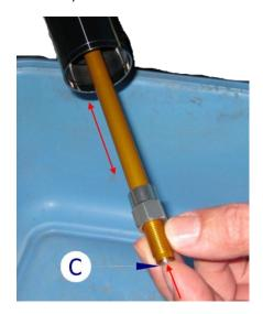
5. Put the fork in a vertical position and insert 250 mL of Oil OJ01 (SAE05). Move the cartridge stem up and down multiple times until the rebound has homogenous braking;
