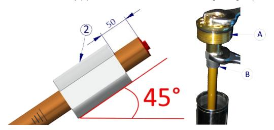
9. Tighten the cap (A) on the tube with a 17 mm combined wrench and a tightening torque of 10/12 Nm.
