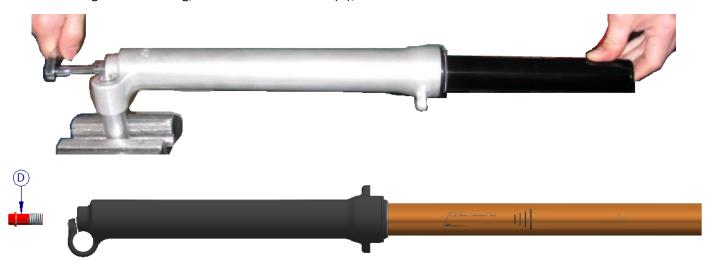
6. Remove the cartridge (E) from the tube. Turn the fork upside down to remove the end stroke cone (F);
