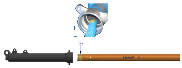
15. Insert the upper bushing (M) and the oil seal support washer (L) on the tube. Push the parts inside with Tool 1 from the side without knurling;
