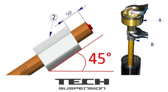
24. Tighten the cap (A) on the tube with a 17 mm combined wrench and a tightening torque of 10/12 Nm.
