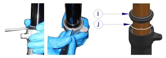
12. Tighten the wheel's axle in a bench wise with aluminium plates and insert the leg on the axle. Forcefully pull the tube out of the leg and remove all parts from the tube (I-N);
