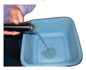
7. Put the fork in a vertical position and insert 250 mL of Oil OJ01 (SAE05). Move the tube up and down multiple times, then push it to the end of the stroke;
