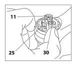
WARNING: NEVER use the closed position of the lever (25) on downhill sections as the hydraulic suspension will not react appropriately to impact with obstacles, causing loss of control of the bicycle and can cause serious or fatal accidents.
