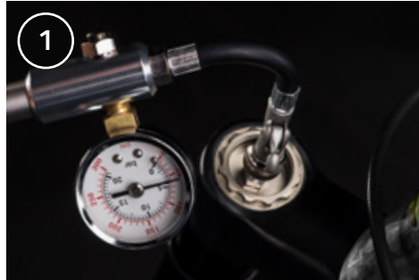
1 Remove the air from the positive chamber using the appropriate Formula high pressure pump.
