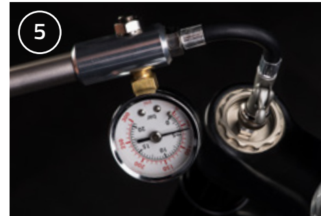
Re-inflate to the desired pressure.
