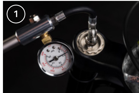
Remove the air from the positive chamber using the appropriate Formula high pressure pump.
