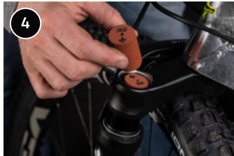
4 Remove the Neopos with your hands or using a 4mm hex wrench by inserting it into the hole.
