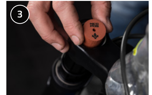
Insert one or more Neopos inside the positive chamber (a maximum of 3 Neopos can be used regardless of fork travel).
