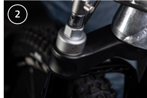
2 Unscrew the positive chamber cap using the tool found in the aftermarket box of your Formula fork.
