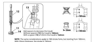
WARNING: The stroke of Selva fork cannot be increased with respect to the max permitted stroke. Component no.7 cannot be interchanged from one
