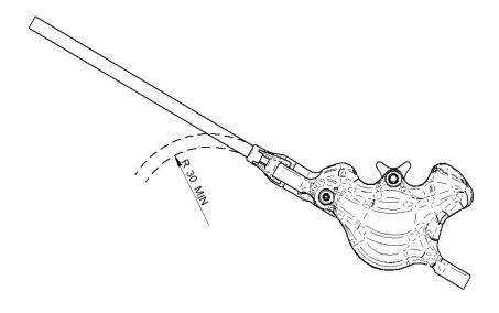
If you need to use a superior curve radius, we advise you to use the specific kit made for it. In case that you didn't respect this warning, it can damage the hose near to the connection at the caliper. Those damages will not be covered by the warranty.
