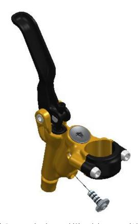
4. Unscrew the lever pivot (7 and 8). Remove the dust seal (9) and the seeger (10), so that the lever and the pushrod can be removed.
