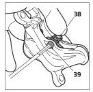
Insert the suitable Formula spacer as shown in the figure.
