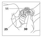
WARNING: NEVER use lever (25) in the closed position when riding downhill since the hydraulic suspension will not work in the proper way in case of obstacles and this may lead to loss of control of the bike and to serious accidents or death.
