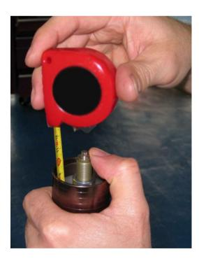
Bring the oil level to 100 mm from upper edge of part F (keep the outer tube and rod, to the end of the stroke).
