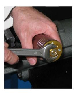
Using a 17 mm open-ended loosen the end plug and screw it completely with torque 11,7 ÷ 13,7 Nm .
