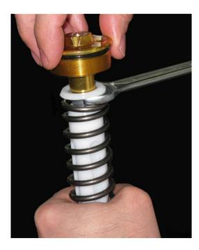
• Screw totally the cap on the rod , as shown in figure .
