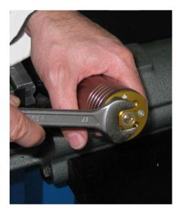
• Using a 17 mm open-ended loosen the end cap and unscrew it completely.
