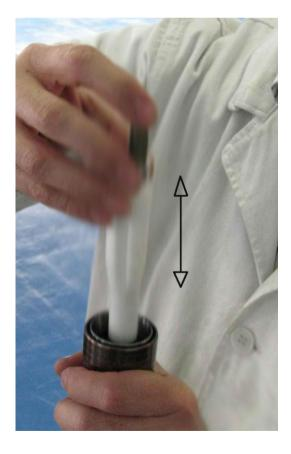
• Using the rod, pump up and down, until you feel smooth braking, on the return stroke.
