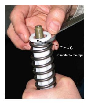
• With the 16 mm open-ended spanner into the lock nut, insert the washer G, making sure that the chamfer is facing the top.
