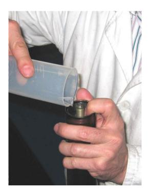
Place the suspension in a vertical position and put some new oil. Cross : Use oil type OJ 01 (SAE 5)
