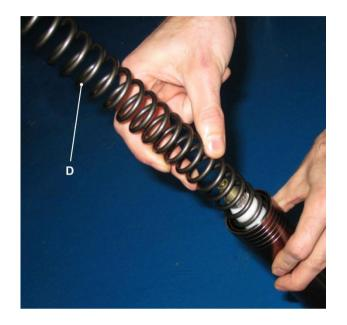
• Insert the spring D in the outer tube, as shown in figure
