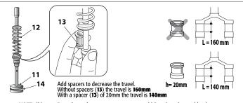
**NOTE:** Shims on Formula catalogue are 10, 15 or 20 mm thick and can be combined to obtain the required size.
