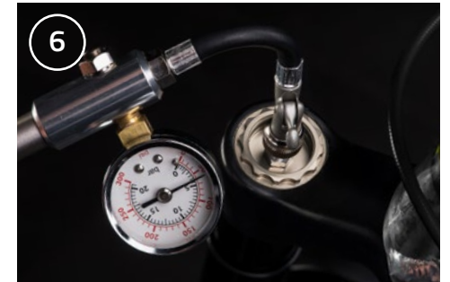
6 Re-inflate to the desired pressure.
