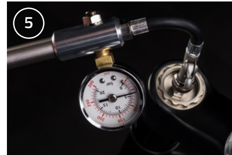
Re-inflate to the desired pressure.
