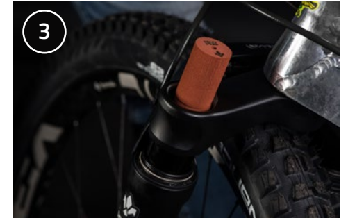
3 Compress the fork until the Neopos is visible.
